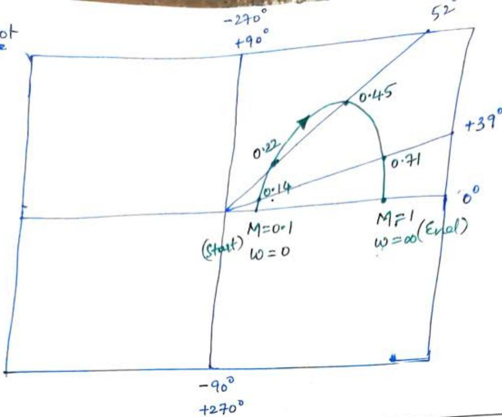
② Draw the polar plots for  $GH(s) = \left(\frac{s+10}{s+1}\right)$  which is T/F of the (LPF, lag compensator)?
