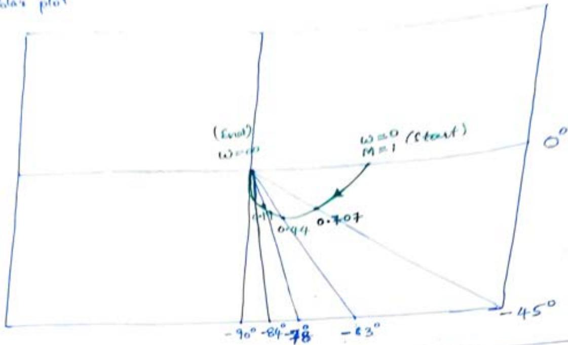
⑥ Draw the polar plot for  $GH(s) = \left[ \frac{s+1}{s+10} \right]$  which is the T/F of (HPF w/ lead compensation)
