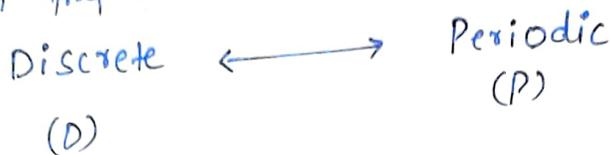
→ In any time domain continuous will be transformed into the non-periodic in freq domain & vice versa.
