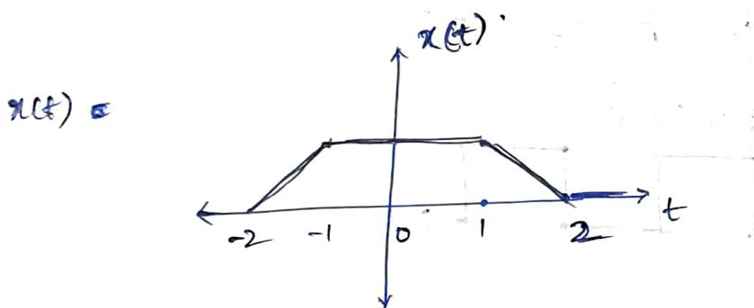
④ Write the following signal in terms of singularity functions
